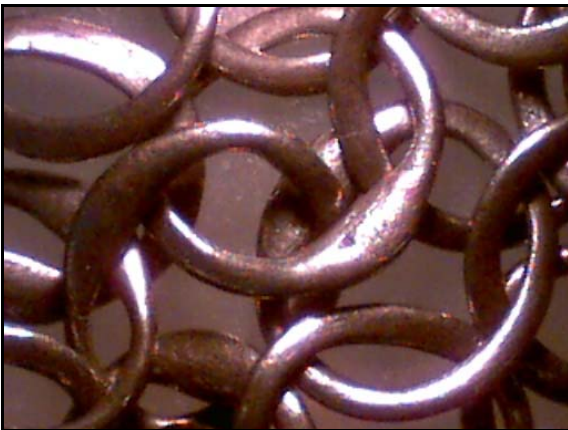
Figure 13. Maille coif back. 15th Century (Sheldon) Back of wedge rivet, barely discernible rectangular rivet back.
