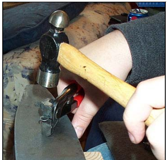
Figure 21. Peening wedge rivet
