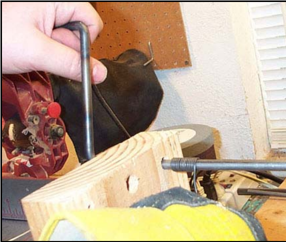
Figure 16. Winding coils on mandrel
