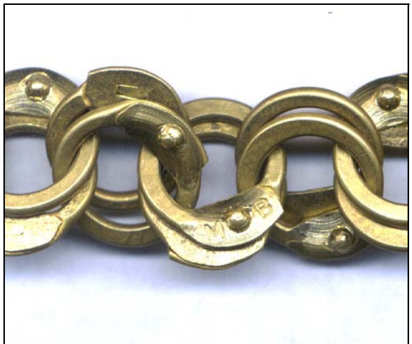
Figure 12. Example of stamped maker's make on Knight's chain.
