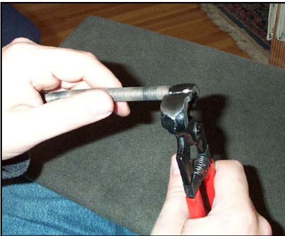
Figure 17. Cutting individual rings w/ overlap
