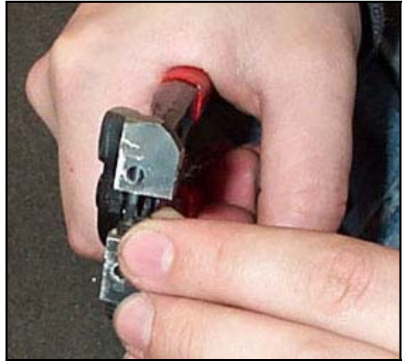
Figure 19. Piercing hole for wedge rivet
